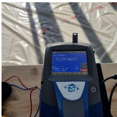
**DustTrak** Aerosole < 1 µm
