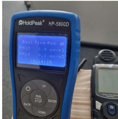
**HOLDPEAK**; Feinstaub 2,5 µm – 10 µm
